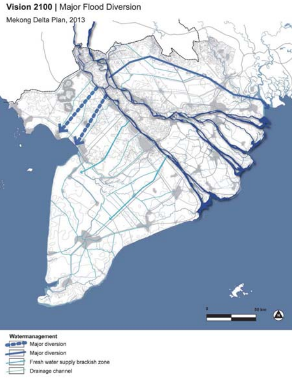
Figure 7-5 Schematic presentation of the principle that large scale additional discharge infrastructure may be required in the future to keep flooding measures in the Middle Delta in control. Systems of canals dug rivers, cascades to bypass the Middle Delta in control, either the West Sea (Gulf of Thailand) through the Long Xuyên Quadrangle or the East Sea through the Plain of Reeds and the Vam Cỏ River. The exact location, dimension and design are still subject for research.
