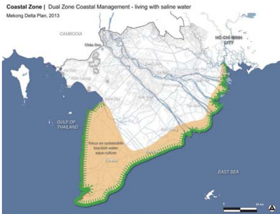
Figure 7-10 Schematic presentation of strategy for water resources management in the Coastal Zone of the Mekong Delta. The Dual Zone Coastal Management strategy assumes a wide Coastal Zone as a first line defence in which a new sustainable brackish water economy has developed. A triplet system of seabass-tilapia-shrimp would form the base of the aquaculture economy, also aiming at restoration of the mangrove coast. A second defence line of dykes would form the separation between the brackish and the fresh water economy and the flood safe defence line. The first defence line is supposed to grow, accrete with sea level rise, the second defence line will bring the high required safety level in the long-term.
