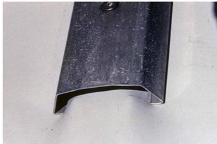
Figure 28: The Carpitech patented anchor-and-tensioning system consisting of 2 stainless profiles pressed onto each other and screwed to the support. A PVC strip will cover the top U profile and will be welded along both edges, to waterproof the anchor.
