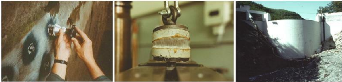
Figure 27: Pull-out tests on adhesive (left), (centre) measurement of traction resistance of a geotextile glued to concrete and Zollezzi arch dam lined with a glued PVC composite (right)
