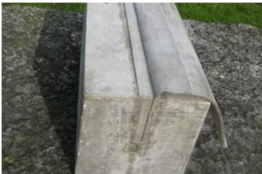
Figure 18: Close-up of a training ‘insert’ fixation (left) and an ‘insert’ on the top of a plastic concrete cut-off (Jibiya dam) (right)
