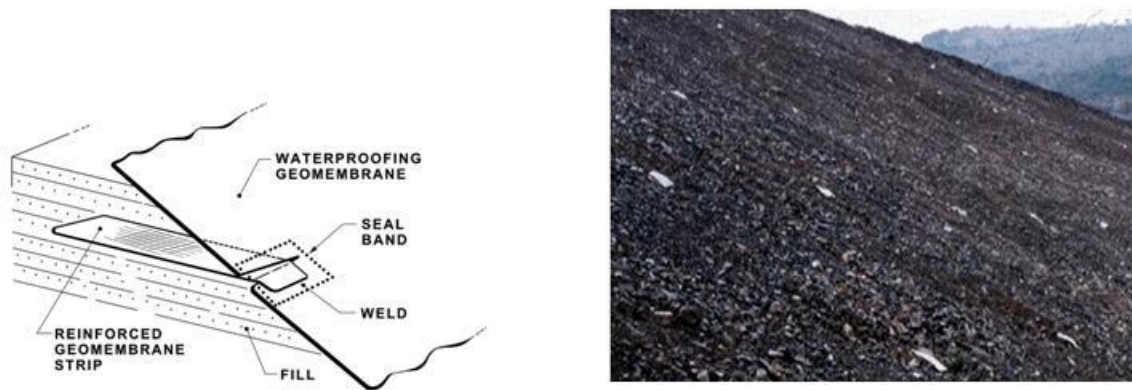
Figure 24: The early concept of anchors in a granular fill (left) and the first such application at Alento cofferdam (Sembenelli [19]) (right)
