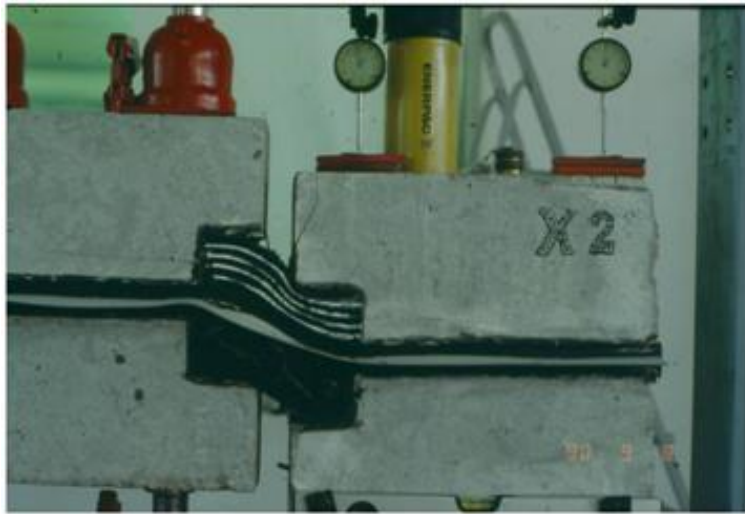
Figure 17: Early tests to cross structural joints with a geomembrane from which the ‘insert’ solution was born
